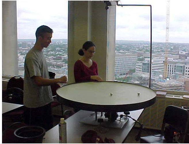
Figure 1: Experiments with ball bearings and dry ice ‘pucks’ on a rotating parabola. A corotating camera views the scene from above.
