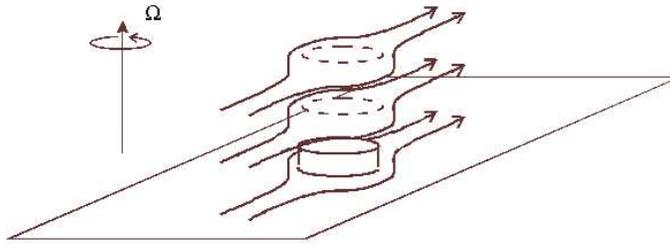
Figure 3-2: This figure illustrates the velocity of the flow relative to the obstacle after the rotation rate of the tank has been slowed slightly. If the relative flow is sufficiently small, the Taylor-Proudman theorem can be applied and Taylor columns will be observed in the flow, as illustrated. Figure taken from 12.307 Notes on the Taylor Column Experiment (2004).
