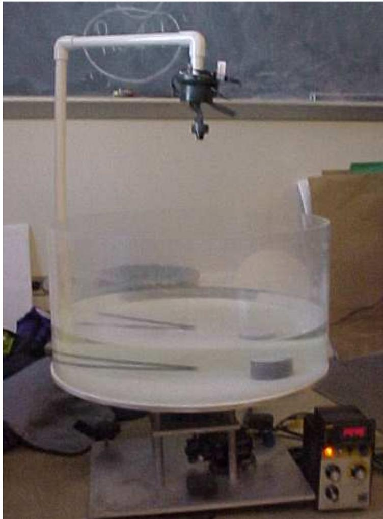
Figure 3-1: This figure shows the setup of the experiment. The tank has a radius  $R=29.6$  cm, and the disk was placed 16.9 cm from the center of the tank. The tank is set to rotate about a vertical axis at a speed of 10.52 rpm. The black lines on the bottom of the tank subtends an angle of  $10^\circ$  and are used in order to estimate the Rossby number for the flow.
