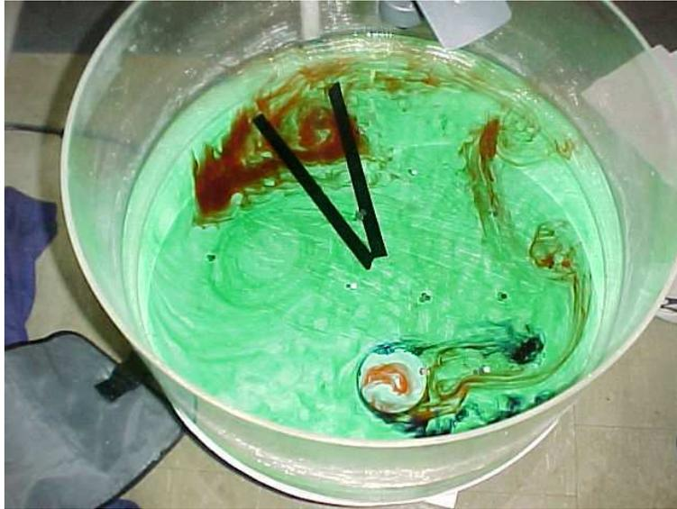
Figure 1-1: The obstacle at the bottom moves slowly through a rotating fluid. Rather than disturbing the flow in all directions, as one would expect, the object pulls a column of fluid parallel to the axis of rotation with it as it moves.
